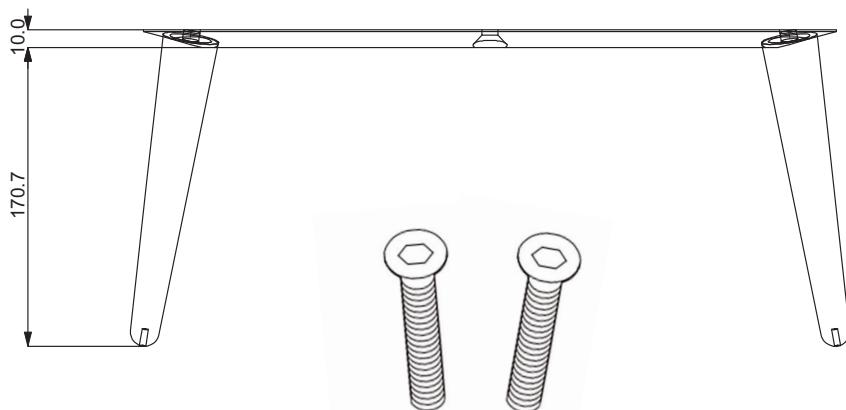
The short countersunk screws are used to attach the CONICA stand to the base of the speakers.
