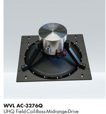
Dimensions: The square frame measures 446mm x 416mm. The AC-3276Q has a 10mm thick front. We recommend mounting from the front with M5 screws. The housing circle cutout is ø392mm and has 3 extensions measuring 28x31mm at 120degree angles. The cone diameter is ø320mm.
