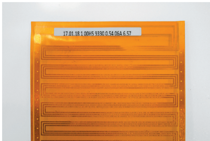
Each diaphragm is recorded in a database and receives an individual label, including a serial number and measured impedance.
