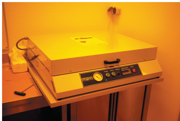
UV exposure unit with vacuum suction of the exposure mask
