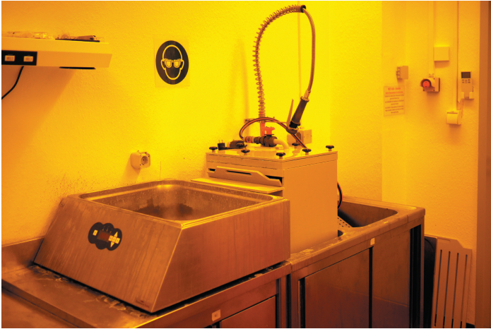
System for developing and washing the exposed film
